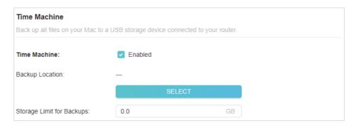
3. Tick the checkbox to enable Time Machine.
