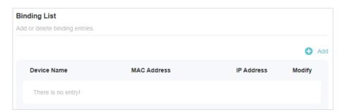
2) Click VIEW CONNECTED DEVICES and select the device you want to bind. The MAC Address and IP Address fields will be automatically filled in.
